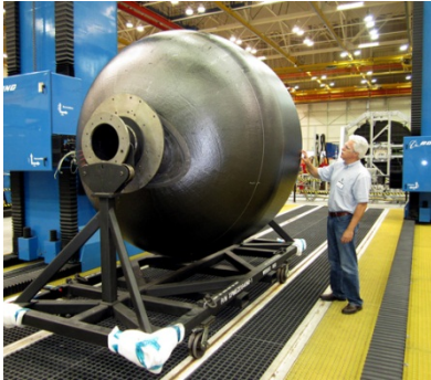
2.4-meter Tank Non Destructive Inspection
