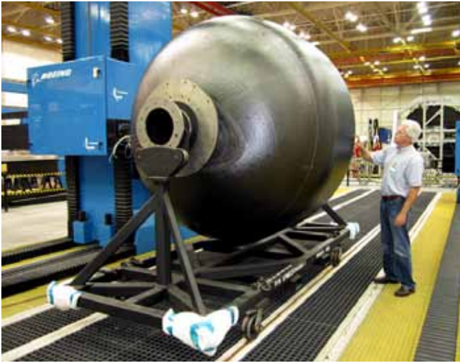
NASA engineer Larry Pelham (right) checks out the 2.4-meter diameter composite tank test article.
