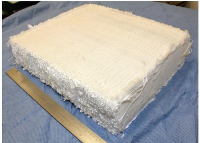
3D woven, quartz-fiber preform (12 x 10.5 x 2.7 in.) prior to resin infusion.
