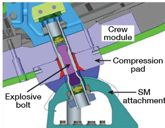
*Expanded view of the compression pad interface with the service module (SM).*
