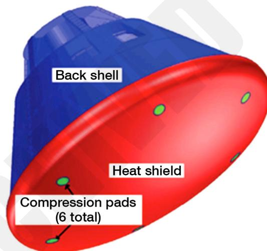
*Orion crew module highlighting the compression pads in the heat shield.*
