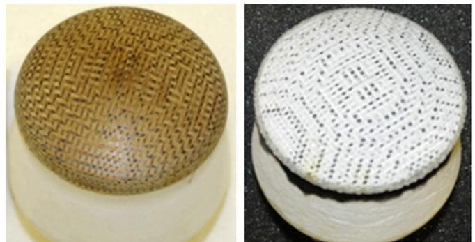
3D quartz cyanate ester arc-jet samples before (left) and after (right) exposure to lunar return-relevant conditions of 750 W/cm<sup>2</sup>.
