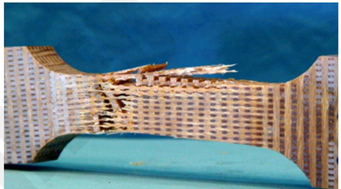
3D-MAT posttest tensile coupon; the 3D composite has superior mechanical performance compared with the current 2D pad material.
