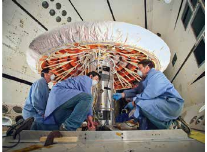
Engineers checked out the Inflatable Reentry Vehicle (IRVE-3) following the complete inflation system test under vacuum conditions in the Transonic Dynamics Tunnel at NASA's Langley Research Center in Hampton, Va.
