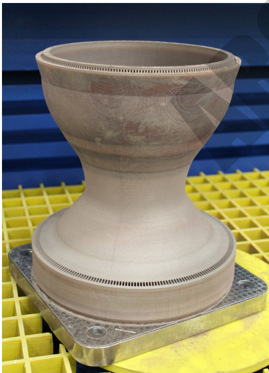
Aft chamber segment of a development unit printed with GRCop-84 demonstrating the ability to print features required for thrust chamber.
