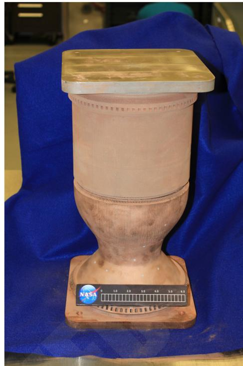
**Full aft and forward chamber segment development units printed with GRCop-84 demonstrating the ability to print features required for thrust chamber.**
