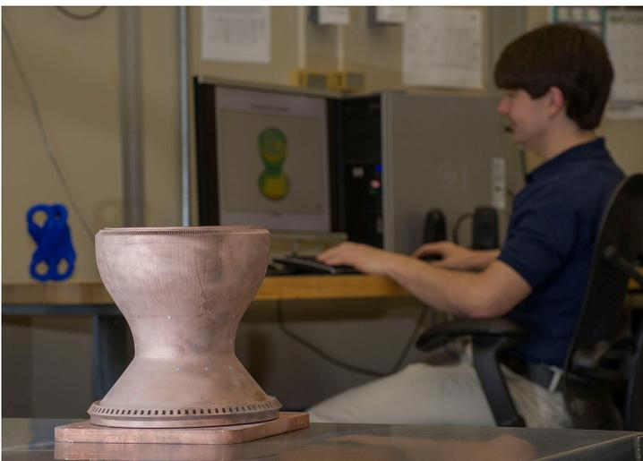
**NASA engineers used 3-D printing to make the first full-scale copper engine part, a combustion chamber liner that operates at extreme temperatures and pressures. Structured light scanning, seen on the computer screen, helped verify that the part was built as it was designed.**
