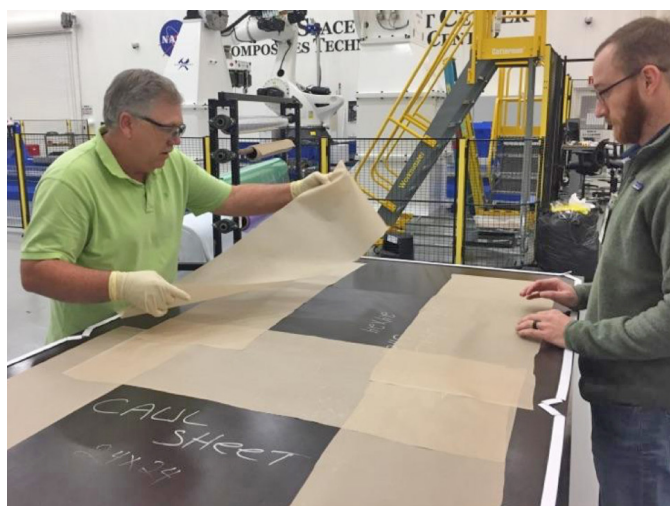
Team members prepare panels for bagging/curing during the fabrication process at Marshall Space Flight Center's Composites Technology Center.
