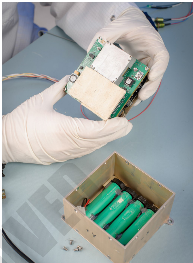
AVA controller is smaller than a stack of 6 compact disc cases, and weighs in at under a kilogram—batteries included!
