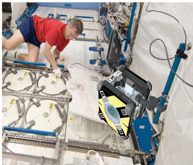
Illustration of an Astrobee robot perched on a handrail to take video of a crew activity.
